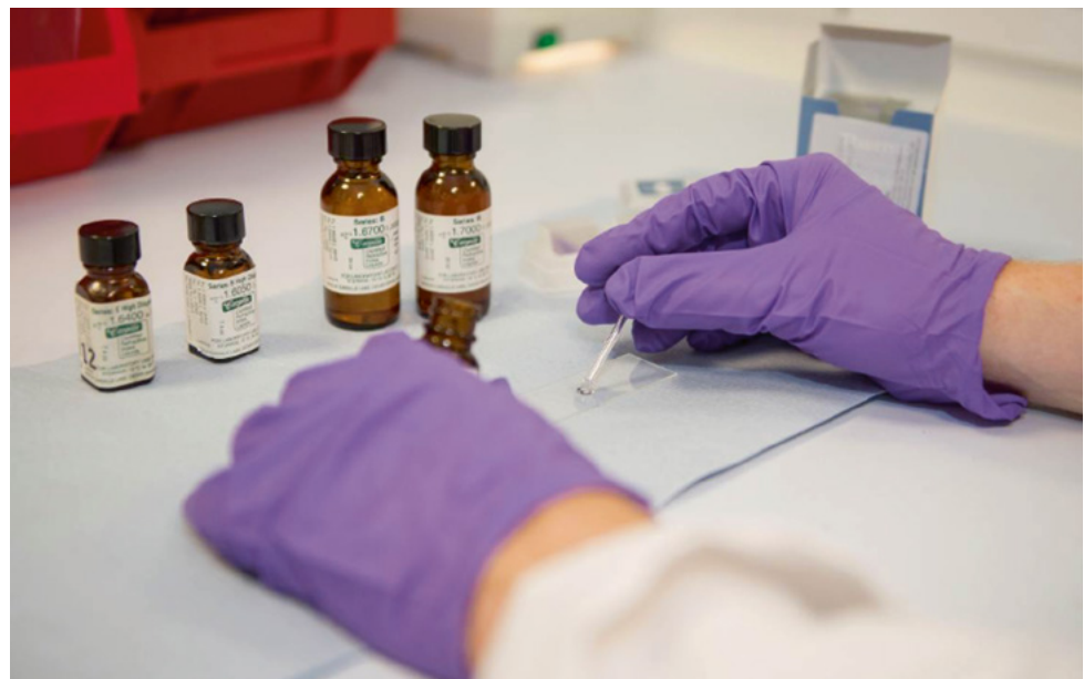
Figure A2.3 RI liquid being placed on a glass slide
