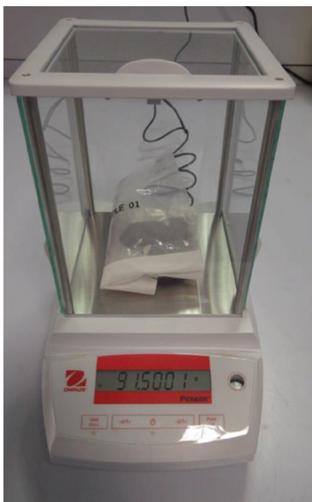
Figure A3.1 Water absorption sample being weighed
