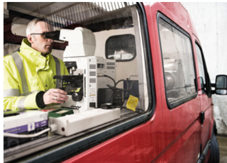
Figure A5.7 Analyst carrying out a PCM count in a mobile laboratory
